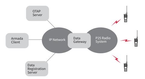
EFJohnson's Armada OTAP implementation is made up of three components: Armada Fleet Management Software, the OTAP Server, and the Data Registration Server:
