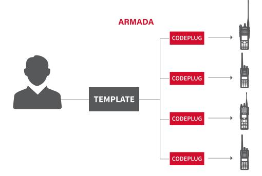
Programs a fleet of radios simultaneously
